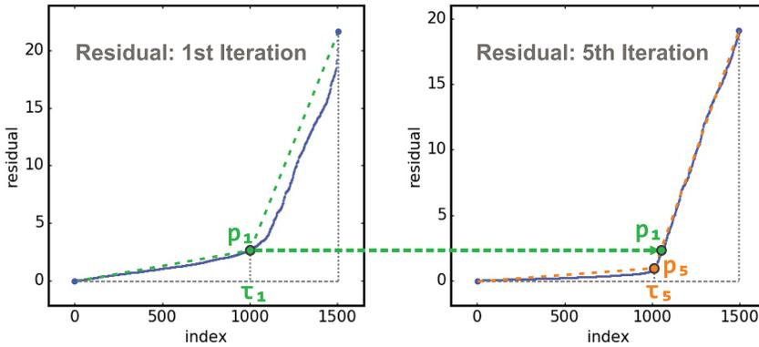
Fig. 2. Residual  $r$  in ascending order for the 1st (left) and 5th (right) iterations of *RHCT* algorithm.
