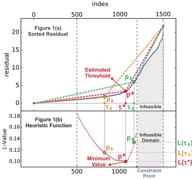
Fig. 1. The blue line in Figure 1(a) indicates the values of residual vector  $r$  in ascending order, and the red point in Figure 1(b) shows the corresponding value of the heuristic function.  $\tau_*$  is the estimated threshold with the minimum  $\mathcal{L}$ ;  $\tau_1$  and  $\tau_2$  are the candidate threshold values in  $\tau_*$ 's left- and right-hand sides, respectively.
